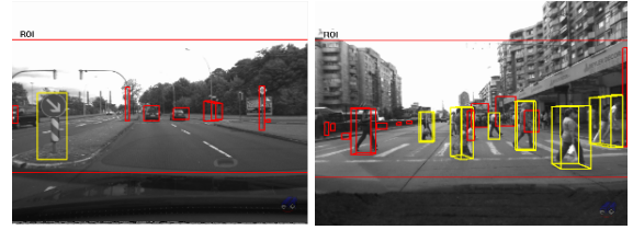
Figure 11: Samples obstacle misclassifications solved by SORT-SGM (pedestrians with yellow color; other obstacles with red color): left image – a false positive; right image – a false negative
